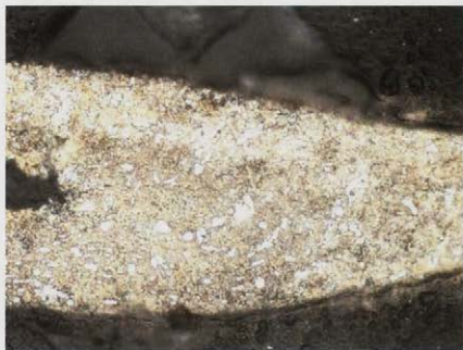
Figure 18 : Recuay animal head : sample from silver colored serrated teeth. The microstructure reveals a heavily worked and annealed gold-platinum alloy matrix incorporating undissolved platinum particles, finely dispersed through the gold. The extensive and very fine scatter of the remnant undissolved platinum particles shows that a considerable attempt has been made to homogenize and disperse the platinum through the gold matrix, resulting in a very silvery colored surface to the composite material. Magnification x490, etched in aqua regia.
