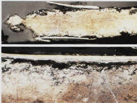
Figure 20a : Unetched cross-sectional view of part of the silver sheet of the spoon with a gold inlay over part of the surface. As polished, magnification x80.
