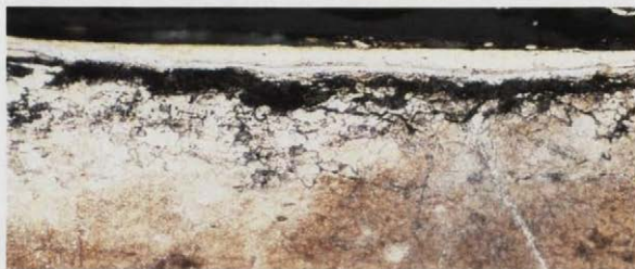
Figure 20b : Etched microstructure showing the diffusion interface at the surface between the gold foil inlay and the silver substrate. The junction appears double because corrosion has only attacked the underlying alloy to a certain depth below the surface, diffusion of gold into the topmost silver layer has resulted in enhanced resistance to corrosion. The silver grains clearly show discontinuous precipitation of copper at the grain boundaries. Etched in acidified potassium dichromate, magnification x320.
