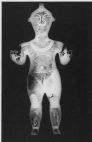
Photograph 9: Radiograph of the standing male lime-flask showing construction details as well as casting faults and secondary casting runs (see text for interpretation) [S. La Niece, British Museum]
